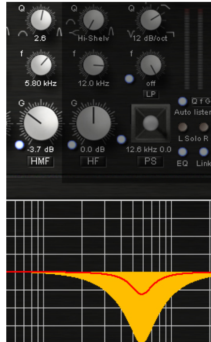
Auto listen "Q" with NEGATIVE gain (see the HMF band gain at (-3.7dB))
